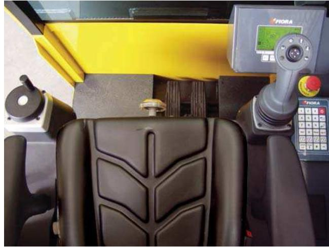
The control centre features a large LCD which displays the actual wheel angles, the selected steering and travel modes of operation.
